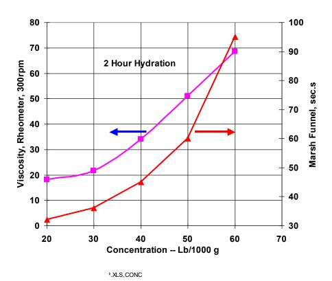
**Figure 1: Viscosity with Concentration** shows fresh water viscosity for a range of concentrations of Rantec **G150** biopolymer.
